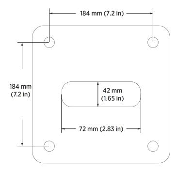
2. Ensure that the conduit stub-up is at the centre of the hole location.
