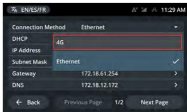
3. To set up station OCPP backend configuration, configure the following CPO settings:
