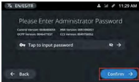
The station password has to be provided by the station owner. If forgotten, you'll have to reset the password and power cycle the station.
