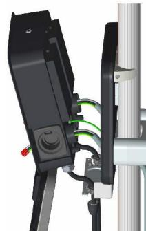
12. Remove four 14 mm M6 screws that secure the grounding plate to the station mounting bracket (c). Remove the grounding plate. When reinstalling the grounding plate, tighten the screws to 16.5 Nm.
