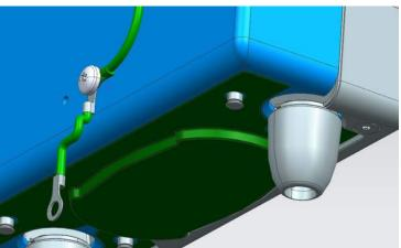
Important: Place the parts in the following sequence wherever a grounding cable is fastened to a part: part (a), washer (b), grounding cable (c), screw (d). This is required to break the anodizing layer and guarantee contact between the bare metal and grounding cable lug.
