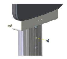
15. Using the thread forming M8 screw and star washer, connect one end of the 635 mm grounding cable and one end of the 241 mm grounding cable to the left (facing the station) M8 hole in the station mounting bracket.
