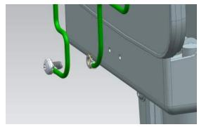
Important: Place the parts in the following sequence wherever a grounding cable is fastened to a part: part (a), washer (b), grounding cable (c), screw (d). This is required to break the anodizing layer and guarantee contact between the bare metal and grounding cable lug.
