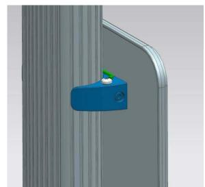
**26.** Connect one end of the 241 mm grounding cable to the CMK column using the thread forming M8 screw and the star washer.
