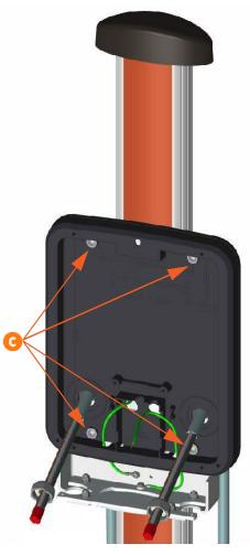
**13.** Remove two 10 mm M8 screws (d) to unfasten the station mounting bracket from the power cable cover.
