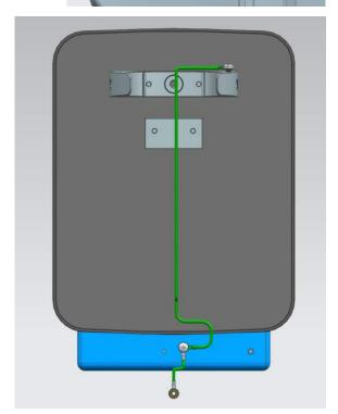
25. Tighten the screw in the CMK clamp end to secure it.
