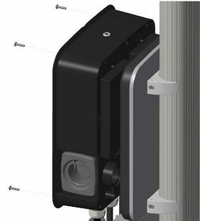
12. Using a 6 mm hex bit, loosen the ends of the clamp ends (c).
