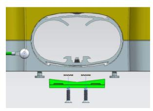
19. Using a 6.8 mm drill bit, drill a hole in the center of the CMK front face, 847 mm from the bottom. Drill the hole between the two holes that are already present.
