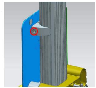
**16.** Remove two M8 screws that secure to the hanger bracket and remove the hanger bracket from the CMK column.
