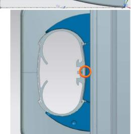
**24.** Using the thread forming M8 screw and star washer, connect one end of the 635 mm grounding cable to the CMK clamp end.
