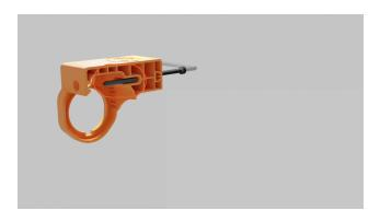
12. Insert the J1772 connector into the repair. Press into place until the guide pin hole aligns with the exit hole.
