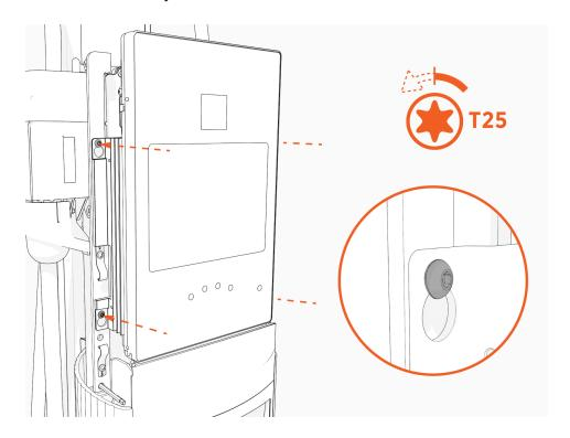
6. Lift the CCOM up and tilt it away from the head assembly.
