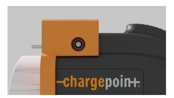
13. Use the hex wrench to tighten the drive bolt. The guide pin slowly extends from the exit hole. If you feel too much resistance but don't see the pin move, check the alignment and try again.
