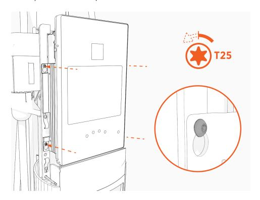
Lift the CCOM up and tilt it away from the head assembly.
