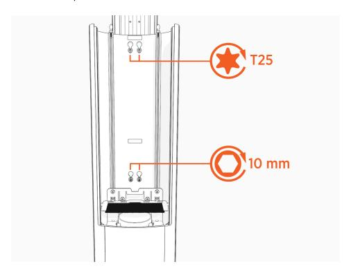
When installing the new CMK, torque the top T25 screws to **5.7 Nm (50 in-lb)**. Use a 10 mm wrench to tighten the nuts near the bottom to **5.7 Nm (50 in-lb)**.
