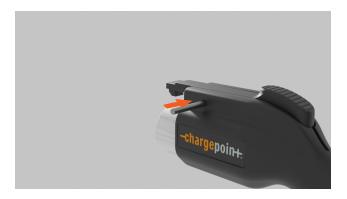
11. Use the hex wrench to loosen the drive bolt. Insert the latch pin fully into the pin slot.
