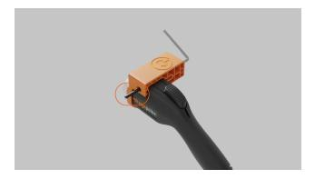
4. Tighten the drive bolt until the latch pin fully extends from the exit hole. Remove it by hand.
