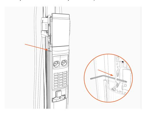
8. Using a T25 driver, loosen, but not remove, four M4 screws that secure the Control and Communications Unit (CCOM) to the head assembly.
