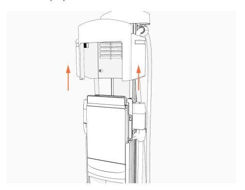
6. Use the L-wrench to loosen, but do not remove, the screws securing the head assembly.
