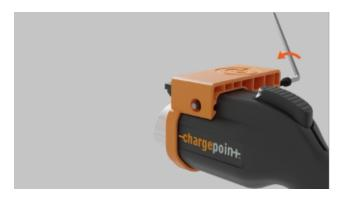
14. Tighten the drive bolt until the guide pin fully extends from the exit hole. Remove the pin by hand. Keep the guide pin so you can use the tool to repair another connector.
