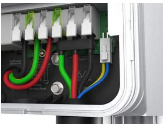
7. Insert the 4-pin plug into the connector to the right of the output supply wiring.
