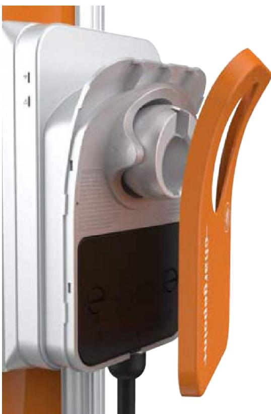
4. Fasten the faceplate to the bottom of the station using two T10 Security Torx screws.
