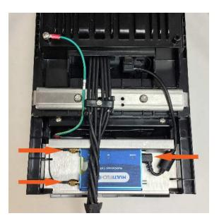
4. Confirm the modem has a SIM card installed and that it is fully inserted. It may be pre-installed and there may be yellow tape over the SIM opening. Do not remove the tape.
