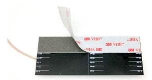
3. Apply the antennas to the back of the head as shown. Press firmly to ensure proper adhesion.
