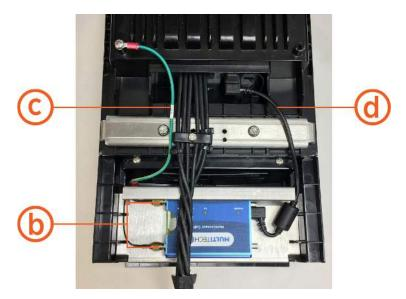
6. Be sure all cables are tucked in behind the bracket to prevent catching on the housing when the head is replaced.
