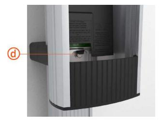
7. Disconnect the blue connector by pressing the side tabs while rocking the connector side to side and pulling downward.
