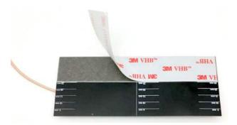
3. Apply the antennas (a) to the back of the head as shown. Press firmly to ensure proper adhesion.
