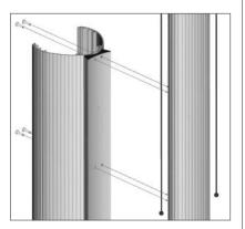
Step 3: Remove the CMK by lifting it about 2" to disengage it from the bottom support nut, then moving it away from the bollard.
