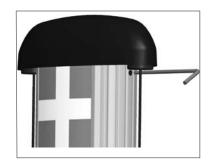
**Step 2:** Each rope is attached to a weight that sits on a shelf. Pull the weight shelf up by pulling the rope located in the middle of the top cap.
