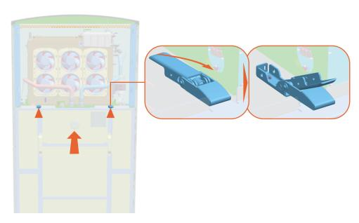
2. Hold the door handles (x2) and tilt out to lift the door off of the flange at the bottom of the door.
