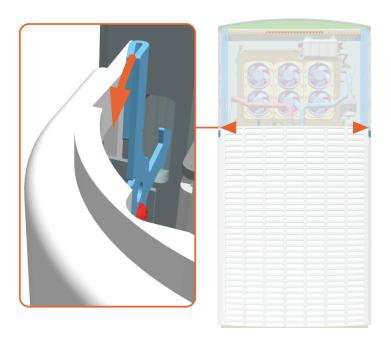
2. While the hook levers (x2) are pulled out, tilt out the panel's upper side to remove.
