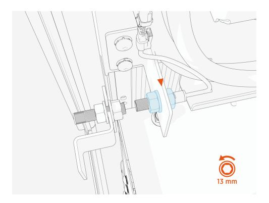
5. Carefully remove the sensor from the bracket.
