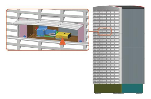
2. Slowly press and push the upper panel sides up to disengage the hooks (x4) behind the panel.
