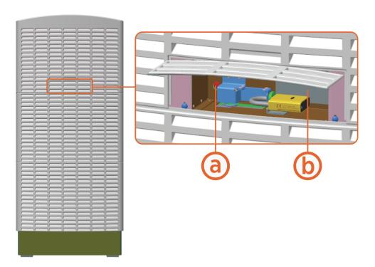
2. The status light (a) must be off (unlit). If the status light is on (glowing any color), do not proceed further with servicing. Wait the required time for energy to dissipate (see safety label (b) on the product).
