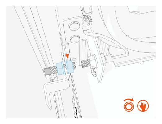
3. Place the washers (x2) and the sensor in its position.
