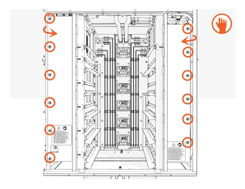
2. Slightly rotate out the edge with the screws.
