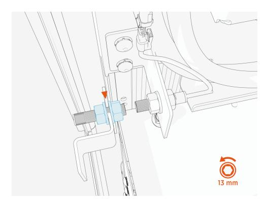
3. Carefully remove the magnet from the bracket.
