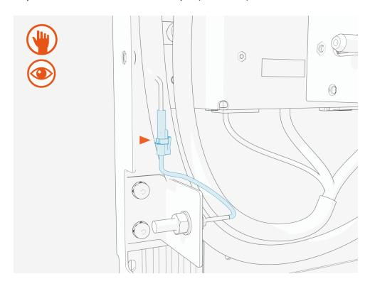
3. Measure the gap (a) between the threaded sides of the sensor and magnet, and ensure the gap is less than 10 mm and as close as possible.
