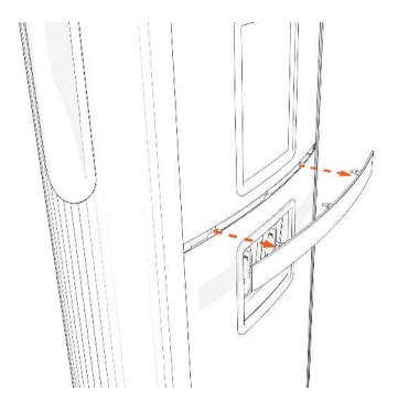
2. Hold the bottom of the holster trim. Pull down, up, and out.
