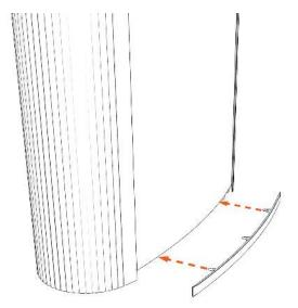
4. Position the upper side of the holster trim onto two hooks. Then press the lower side of the trim into place. **Note:** The holster trim has a specific orientation wherein its upper and lower sides are not interchangeable.
