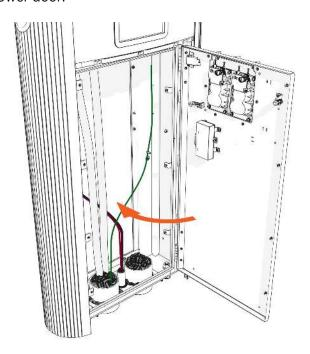
2. Reinstall the lower door screws. Torque to 4.5 Nm (40 in-lb).
