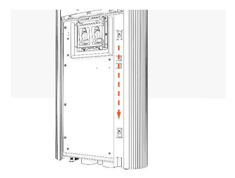
5. Torque screws on the door bracket to 1 Nm (10 in-lb).
