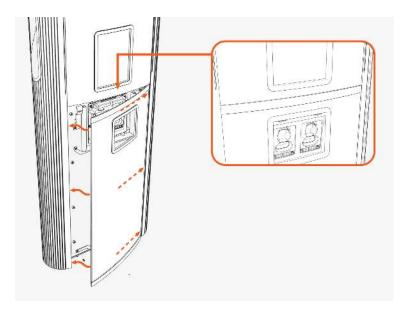
2. Check the top and bottom corners of the cover to ensure they are seated in the side grooves. Then slide the cover down while pressing in on the lower edge of the holster trim and lower edge of the cover to engage the hooks behind the cover.
