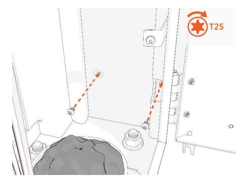
3. Locate two empty screw holes on the lower left inside wall of the Power Link.
