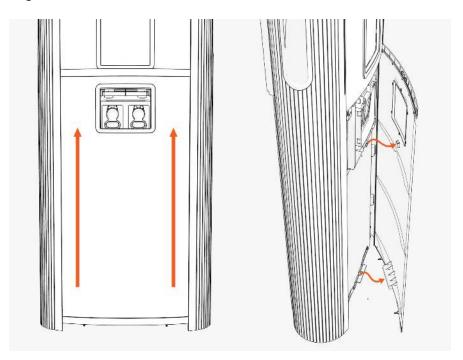
4. Push inwards along one side of the cover to release it from the side groove. As the cover bows out, grip the cover at its top edge. Pull the cover away out and away from the other side groove.
