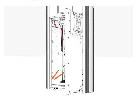
4. Install two screws to secure the left side panel. Hand-tighten.
