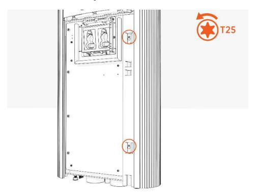
2. Slide the door bracket upwards.
