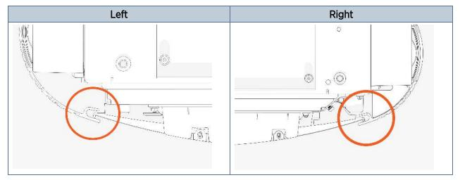
3. Slide the lower cover up. While sliding up, press on the lower edge of the holster trim and lower edge of the cover to release the hooks behind the cover. Remove the cover.
