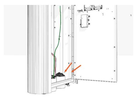
2. Install two screws to secure the right side panel. Hand-tighten.
