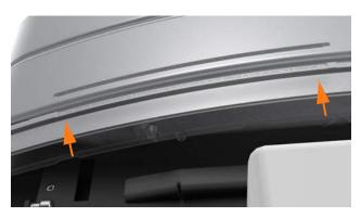
8. Place the two adapter skirts around the edges of the adapter, aligning the tabs of the skirts with the tabs on the base. Use a T25 Torx driver and the four adapter skirt screws to fasten the adapter skirts. Torque to 4 Nm (35.4 in-lbs). When the final cover panels are installed at the end of the *Express 250 Installation Guide*, they fit over the outside of the
