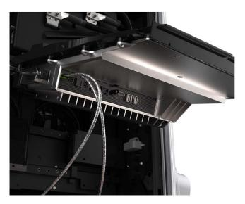
8. Using two hands, remove the panel by firmly pulling it upward to release the guide tabs from the corresponding slots on the Express 250's frame.
