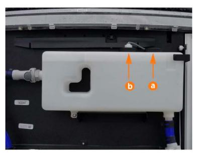
4. Use a funnel to fill the reservoir to the marked MAX line with coolant.
