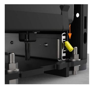
7. Using two hands, squeeze the Power Module mechanism's release bar and lower it halfway to check alignment with the ports and guide posts.
