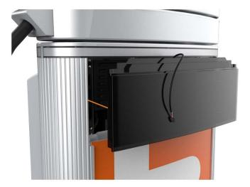
4. When the LED display assembly is released, disconnect the five cables from the back.
