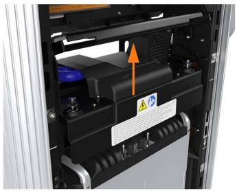
3. At the bottom right of the station, press and hold the yellow release latch while pulling the Power Module tray out of the station completely.
