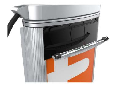
3. Push the LED display upward to release its guide tabs from their corresponding slots on the Express 250's frame.
