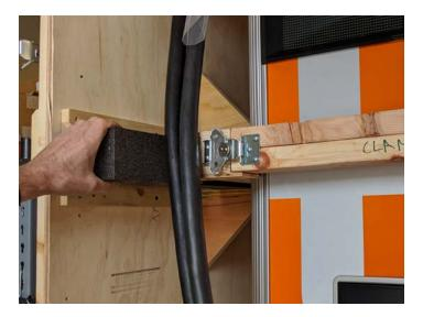
5. Unclamp and open the middle rear retaining beam. Remove the beam and set it aside.
