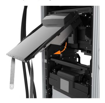
6. Allow the touchscreen to return to its lowest position vertically. Rotate the retention knobs clockwise to retighten.
