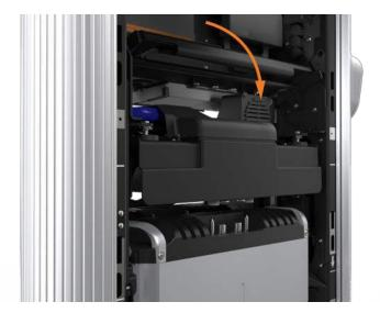
8. Lower the Power Module mechanism until you hear a click as the mechanism locks into place. Ensure the mechanism is fully engaged with all Power Module connectors. The Power Module mechanism should fully cover the ridges on the Power Module's top edge.
