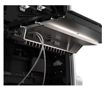
11. With hand pressure, swing the touchscreen down. Loosen both retention knobs (a), allowing the touchscreen beam (b) to slide up vertically. Re-tighten the knobs at the highest position.
