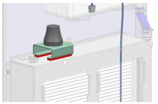
21. Use a zip tie to secure the wiring to the side of the heat exchanger.
