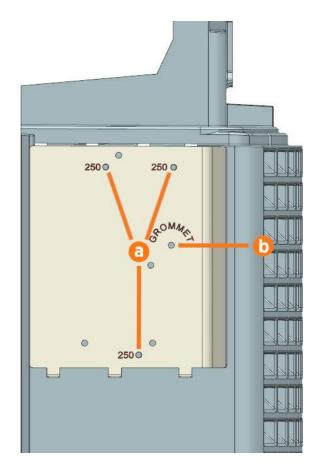
12. Insert the grommet into the drilled opening.
