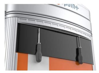
2. Disconnect the power cable that connects the area light bar to the LED display assembly. Remove the area light bar.
