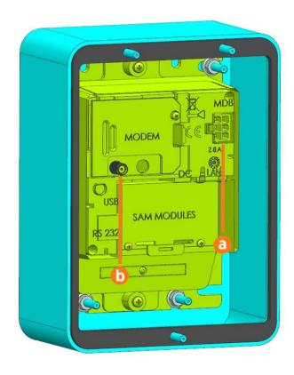
16. Fasten payment terminal assembly to the cover panel. Torque to 2 Nm (18 in-lb).
