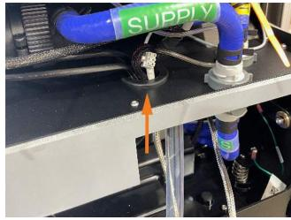
6. Lay the cable on the shelf and hanging off the left side.
