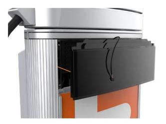
2. When the LED display assembly is released, disconnect the five cables from the back.
