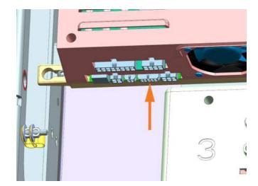
3. Pull the cable down through the top opening on the left side of station frame alongside the other cables.
