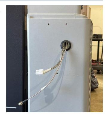
15. Connect the auxiliary power supply (a) and antenna (b) cables to the payment terminal assembly.
