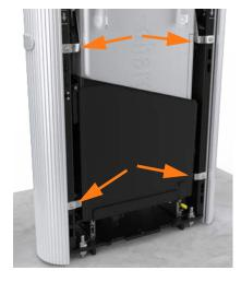
• If front and rear EMI shields are present, use a T25 Torx driver to remove the screws and washers holding each shield over the closed Power Module holder. The rear shield might be in one or two parts, depending on system generation.
