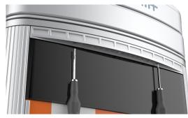
**3.** Disconnect the power cable that connects the area light bar to the LED display assembly. Remove the area light bar.
