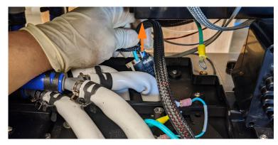
**12.** Unplug the third connector from the **Power Module** port in the Station Management Unit above the module mechanism.
