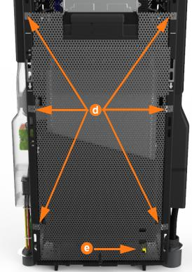
2. Using two hands, squeeze the Power Module mechanism's release bar against the flange. Raise the bar to fully rotate the Power Module mechanism upward to the lock position. Ensure the mechanism has fully cleared the ports and guide posts on the Power Module(s).
