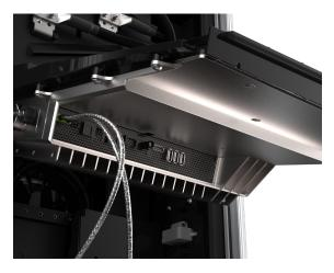
8. Using two hands, one on each side of the middle vent panel, remove the panel by firmly pulling it upward to release the guide tabs from the corresponding slots on the Express 250's frame.
