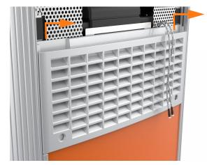
9. Remove the bottom front panel by lifting upward from the bottom of the panel to release the guide tabs from their corresponding slots on the Express 250's frame.
