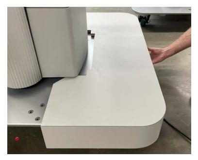
Note: When installed correctly, the sides of the dolly cover are aligned with no visible gaps.
