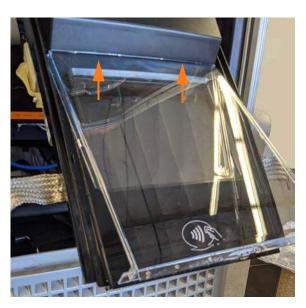
**12.** Align the left and right tab and slot features halfway down each long side of the lens. Ensure the tabs and slots click together.
