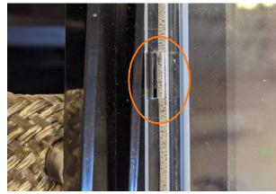
**13.** Gently snap the bottom tabs of the new lens into place. Ensure the tabs and slots click together. Gently test secure placement.
