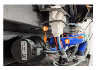
2. Use a right-angle #1 Phillips screwdriver to gently loosen the screw on the clamp bracket (b) until the pump is free to rotate.
