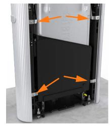
• If front and rear EMI shields are present, use a T25 Torx driver to remove the screws and washers, while holding each shield over the closed Power Module holder. The rear shield might be in one or two parts, depending on system generation.
