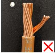
**e.** Verify that no strands of the wire were cut off to fit into the available terminal space.
