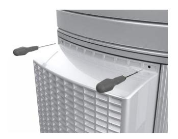
4. Using two hands, lift the middle rear panel straight up and out to disengage the guide tabs.
