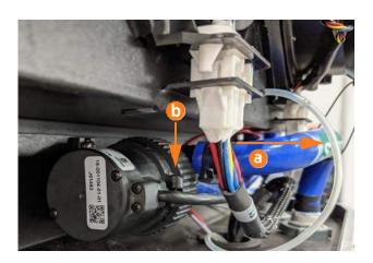
2. Use a right-angle No. 1 Phillips screwdriver to gently loosen the screw on the clamp bracket (b) until the pump is free to rotate.
