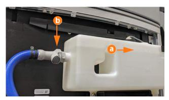
Check the two quick disconnect valves found on either side of the coolant reservoir (b and c). Hold a cloth around the valve and perform a push-pull test at the circled locations to ensure that both of them are firmly seated.
