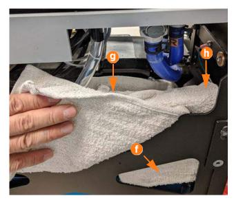
6. Holding the valve with an absorbent cloth, disconnect the supply line below the coolant controller shelf (i).
