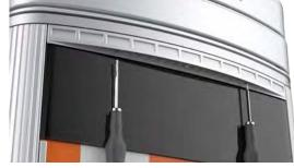
Disconnect the power cable that connects the area light bar to the LED display assembly. Remove the area light bar.
