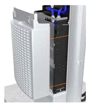
5. Using two hands, one on each side of the lower rear panel, carefully pull the panel upwards to release the panel's guide tabs from their corresponding slots on the Express 250's frame.
