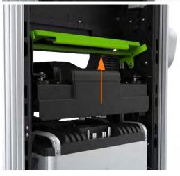
3. If present, use a T25 Torx to remove the front and rear M5 screws and washers attaching the Power Module holder (a) and Power Module (b) ground straps to the Express 250 frame (eight screws in total). Keep the screws and washers for use in a later step.
