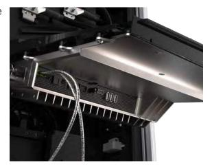
9. Using two hands, one on each side of the middle vent panel, remove the panel by firmly pulling it upwards to release the guide tabs from the corresponding slots on the Express 250's frame.
