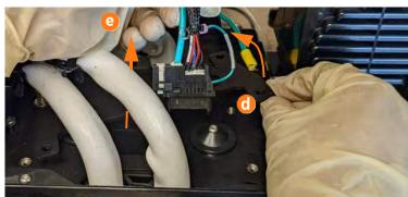
**11.** Lift the rear connector free of the module mechanism.
