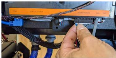
Note: Press in on the connector's rear tab to release it.
