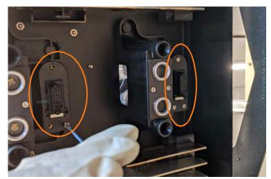
4. Pull each cable connector down and away from its housing. Push upwards on the white plastic latch (a) to unlock the connector from its sheet metal plate (b).
