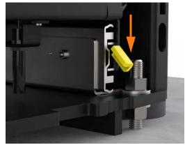
**6.** Rotate both Power Module holders onto their kickstands to provide access to the communication cables.
