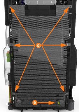
2. Using two hands, squeeze the Power Module mechanism's release bar against the flange. Raise the bar to fully rotate the Power Module mechanism upwards to the lock position. Ensure that the mechanism has fully cleared the ports and guide posts on the Power Module(s).
