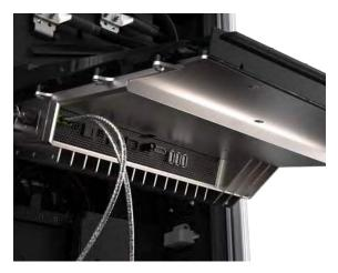
8. Using two hands, one on each side of the middle vent panel, remove the panel by firmly pulling it upwards to release the guide tabs from the corresponding slots on the Express 250's frame.
