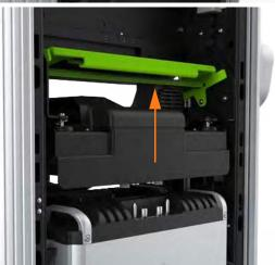
3. If present, use a T25 Torx to remove the front and rear M5 screws and washers attaching the Power Module holder (a) and Power Module (b) ground straps to the Express 250 frame (eight screws in total). Keep the screws and washers for use in a later step.
