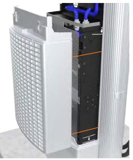
5. Using two hands, one on each side of the lower rear panel, carefully pull the panel upwards to release the panel's guide tabs from their corresponding slots on the Express 250's frame.
