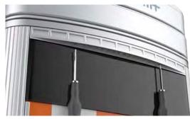
Disconnect the power cable that connects the area light bar to the LED display assembly. Remove the area light bar.
