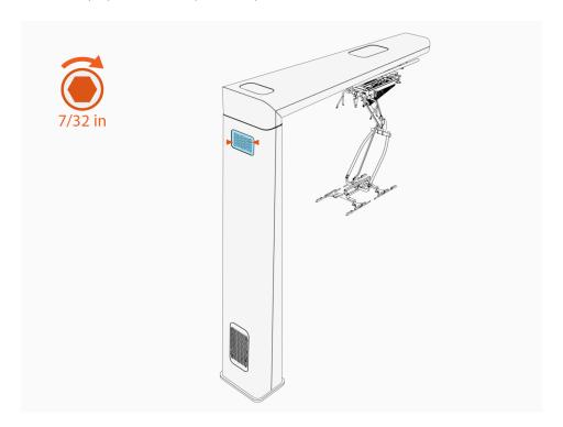
11. Find the lower rear vent panel. Identify the side of the panel with two brackets. This is the rear side of the panel (the panel side that installs facing inside the mast).
