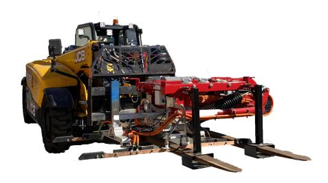
2. Lift and transport the pantograph to its intended position at the mounting rails. Slide the rail clamps to align clamp tabs to the pantograph mounting tabs.
