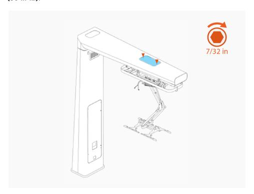
2. Install the hinge access cover. Secure with 3/8 in button-head screws (x2). Torque to **5.6 Nm (50 in-lb)**.
