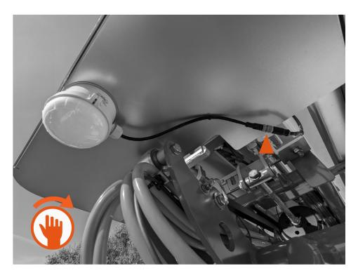
3. Use a zip tie looped through a hole in the front cover to secure the cable.
