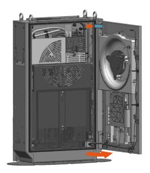
3. Slide the bus bar safety cover up to remove from hooks (x2) and latches (x2).
