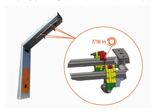
2. Slide and position the two front clamps forward of where the pantograph will mount. Slide and position the two rear clamps behind where the pantograph will mount.
