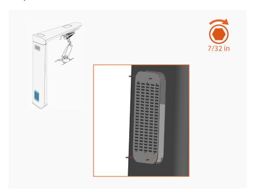
14. Install door window cover. Secure with M4 screw and M4 oversized washer (x10 each). Torque to 1.1 Nm (10 in-lb).
