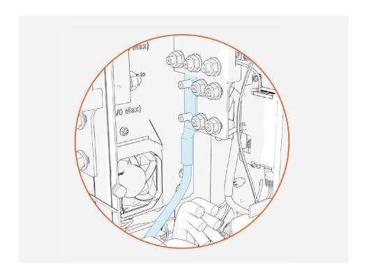
4. Reinstall and tighten the lug nuts.
