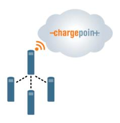
A single gateway station can provide the communications link for up to 24 "non-gateway" stations. One could think of a gateway station as a communications hub. Non-gateway stations must be located within 100' of a gateway station.
