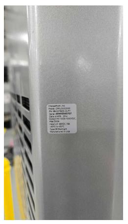
Power Block serial number is located behind the upper front door on the frame in the middle:
