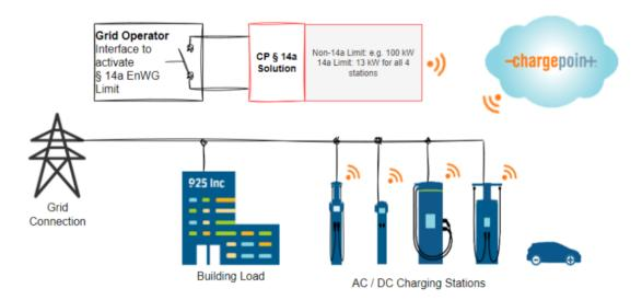
For this purpose, the ChargePoint network control package, consisting of router with antenna and power supply, must be installed and connected to the potential-free contact of the FNN control box or the network operator's ripple control receiver (xxx), see the following diagram.
