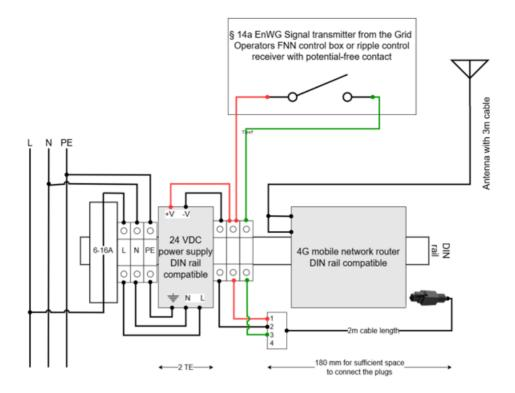
As soon as the signal from the grid operator is received, the total power of all active charging processes is reduced in accordance with the regulatory requirements. The charging stations are regulated to the corresponding limit value, which can also depend on other controllable consumption devices in accordance with Section 14a. The ChargePoint grid control package thus fulfills the requirements of §14a EnWG and entitles the user to benefit from reduced grid charges.
