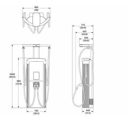
Express Plus Power Link 2000, with liquid-cooled cable, single connector
